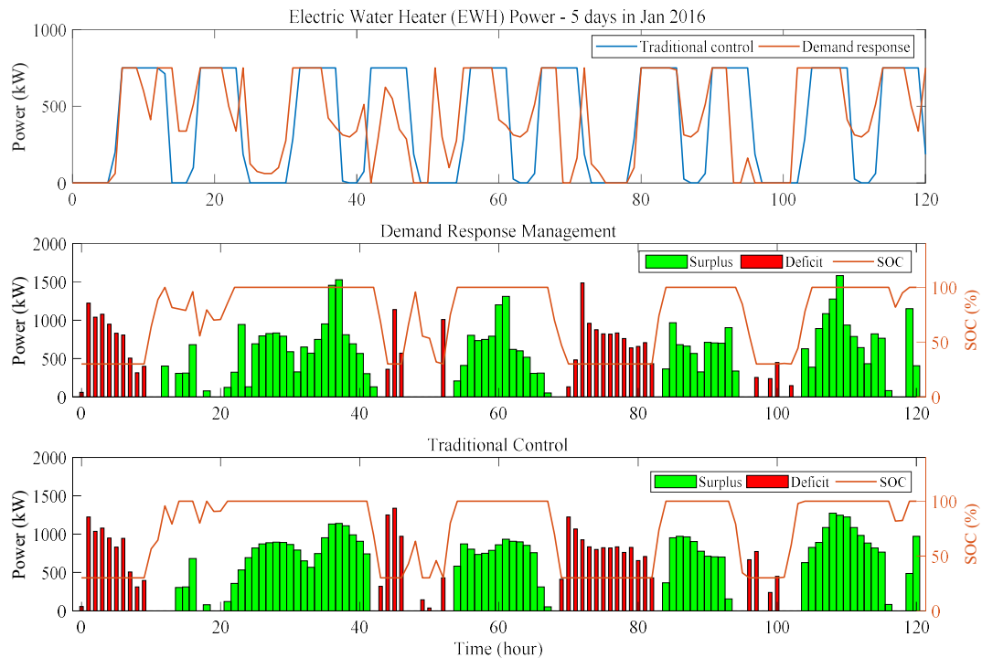
Figure 40: Performance of the EWH demand response controller in comparison to the traditional controller for 5 days in January.
