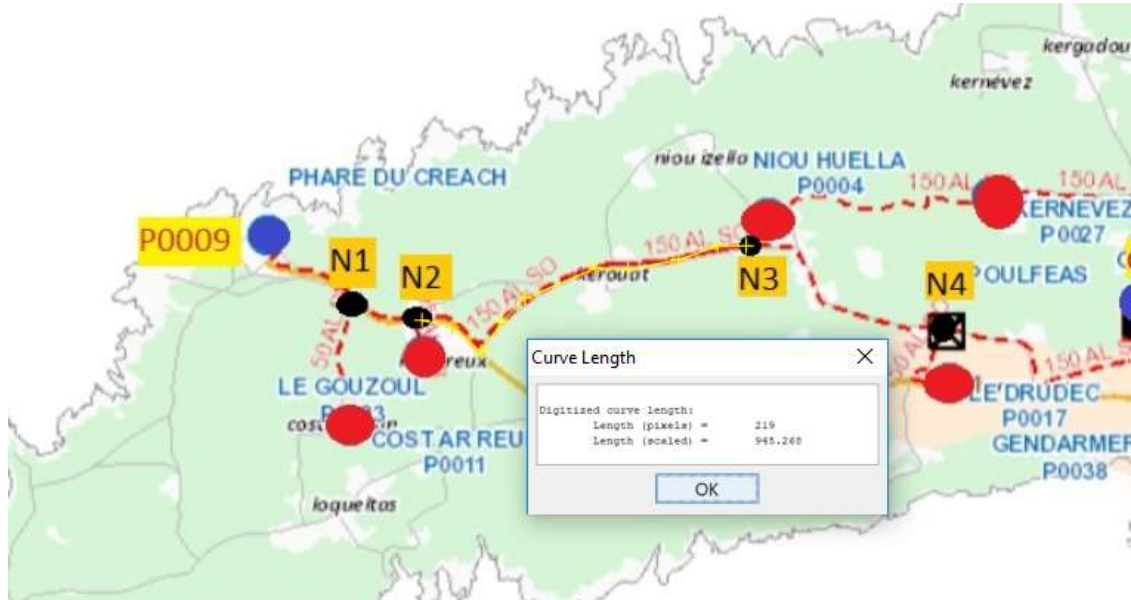
Figure 43: Example of estimating the cable length employing PlotDigitizer software
