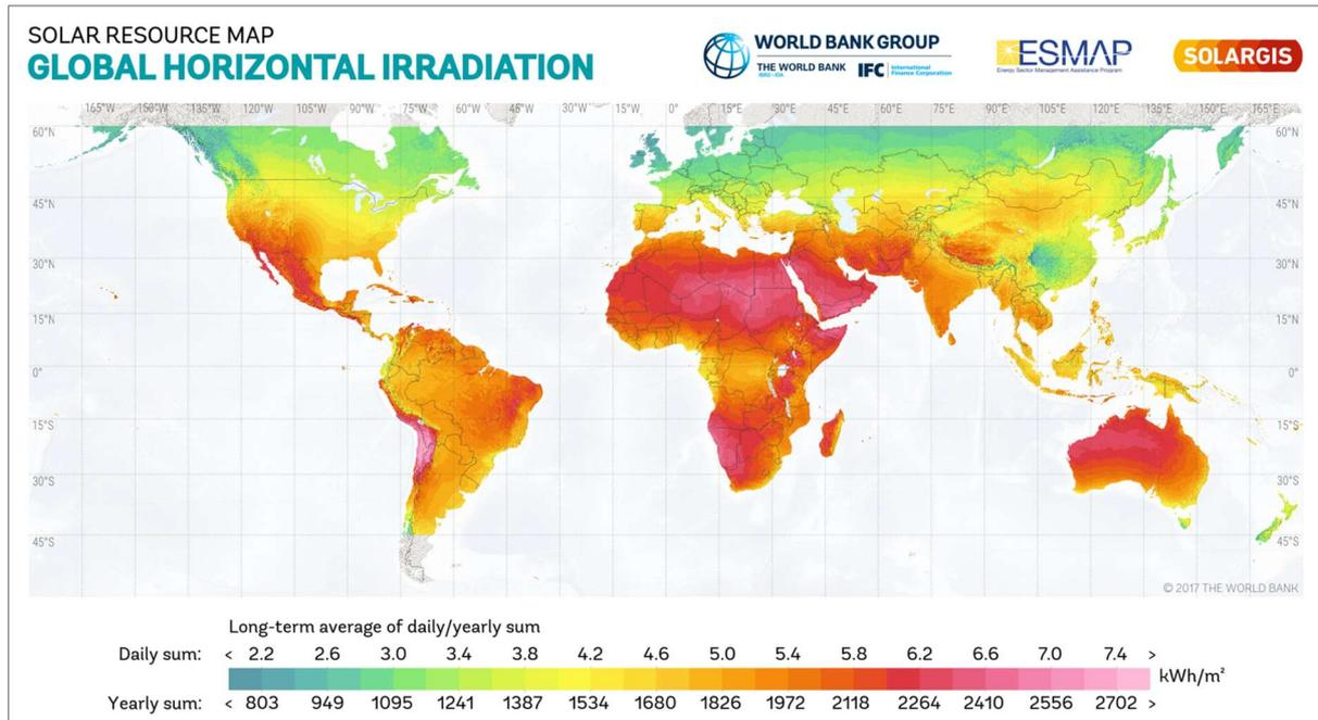
**Figure 3-2:** Map of global horizontal irradiation (source: SolarGIS, 2018)
