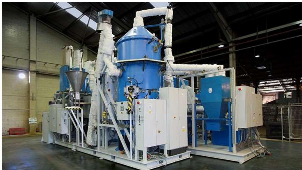
Figure 3-9: The Plaxx RT7000 processor for converting mixed plastics into fuel (source: Recycling Today, 2017)
