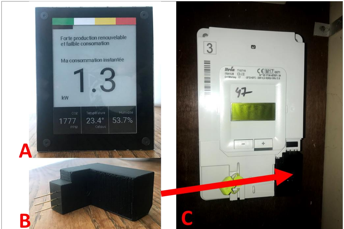
Figure 1 : Photos of the display (A), the data gathering module (B), and the module installed on the Linky Smart-meter (C)
