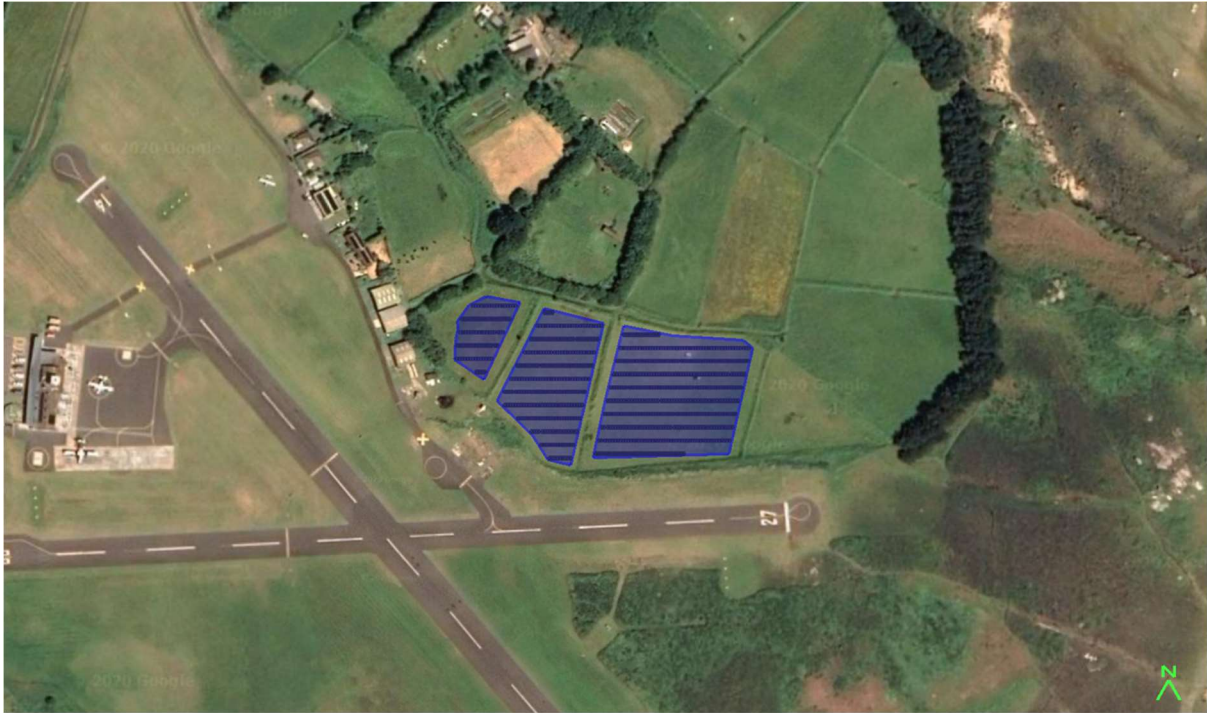
Figure 16 - The three segments shown use area that was deemed appropriate by GIS analysis, and provides adequate land space for the 480kW solar. From left to right the segment areas are 1265.7m 2 , 3783.6m 2 and 6313.2m 2 , totalling 11,362.5m 2 of land. The 1,600 solar PV modules are angled at 34 degrees and the module pitch length (row spacing) is 6.6m.
