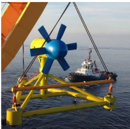
Figure 7. Turbine Sabella D-10 In-stream marémotrice.
