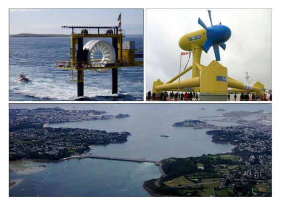
**Figure 3-3:** Examples of tidal power technology: OpenHydro turbine deployed at EMEC (Source: OpenHydro, 2018) (top left); Sabella D10 turbine (Source: Open Ocean, 2015) (top right); La Rance tidal power plant (bottom).
