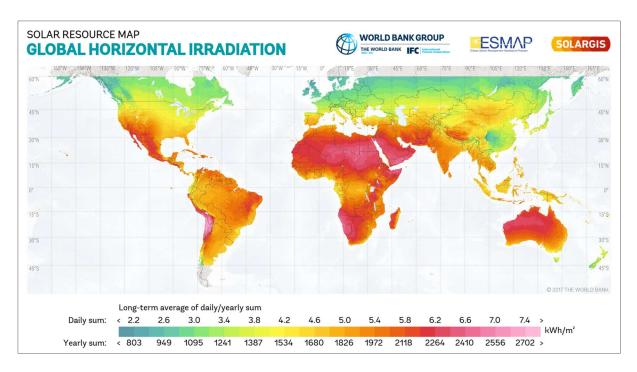
Figure 3-2: Map of global horizontal irradiation (source: SolarGIS, 2018)
